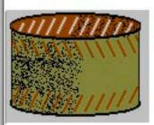
The small cans included in the meal were ideal for making a stove. Using a "John Wayne" pierce a series of closely spaced holes around the top and bottom rims of the can. This stove was satisfactory, but did not allow enough oxygen to enter which caused incomplete burning of the blue Trioxin heat tablet, causing fumes which irritated the eyes and respiratory tract. A whole heat tab had to be used.
